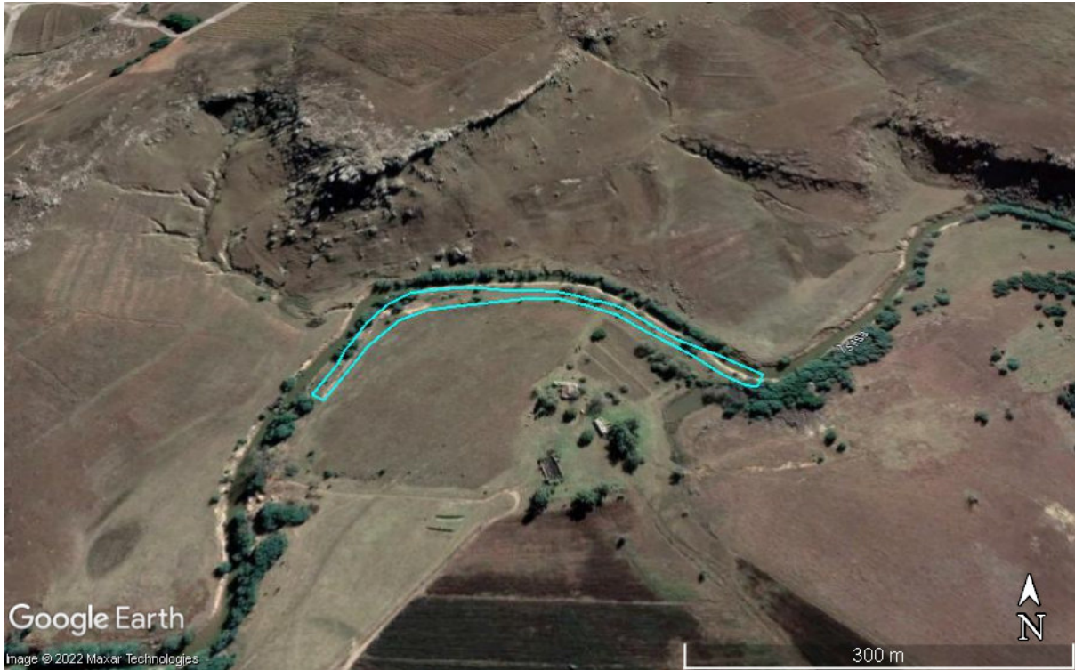
Figure 2: Google Earth map for the proposed stretch along the Tsitsa River that will be mined for sand (turquoise band).
